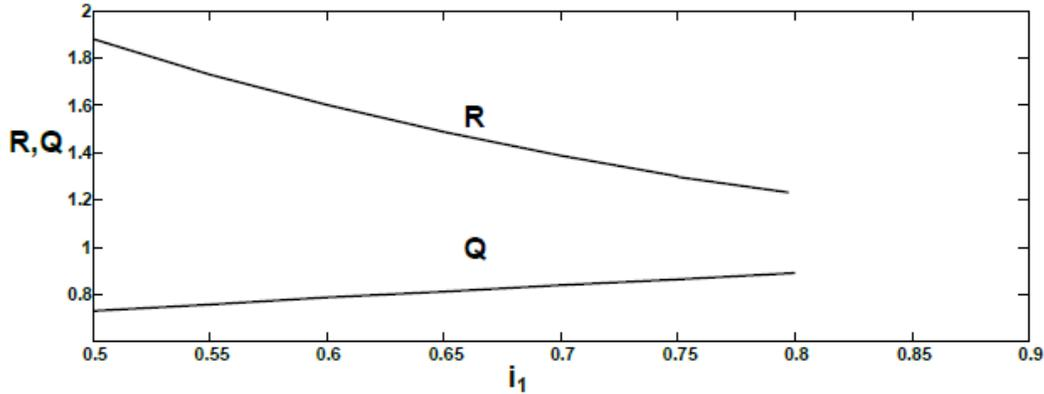
Fig. 8. Effect of the material density at the inner surface on the energy absorption ( $R$ ) and weight ( $Q$ ) for  $a/b = 0.5$ . The mass density at the outer surface is kept constant  $i_2 = 0.4$ . The energy absorption and weight are normalized by those in a homogeneous cylinder with  $i_3 = 0.6$ .
