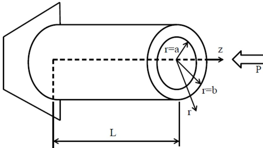
Fig. 4. Formulation of the problem: Foam cylinder between constrained within rigid enclosure formed by inner and outer walls protecting foam from external side loads and environment is subject to axial loading. By varying the mass density and stiffness from the inner to outer radius significant energy can be absorbed by a relatively light structure.
