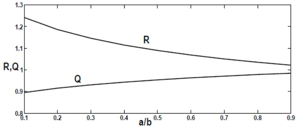
Fig. 7. Energy absorption ( $R$ ) and weight ( $Q$ ) in a functionally graded cylinder ( $i_1 = 0.7$ ,  $i_2 = 0.5$ ) normalized by the energy absorption and weight in a homogeneous cylinder ( $i_3 = 0.6$ ) as functions of the inner-to-outer radii ratio.
